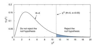
Principles of a  $\chi 2$ -test. The null hypothesis that the two distributions are identical cannot be rejected if the measured  $\chi 2$  is lower than the critical  $\chi 2$ .
