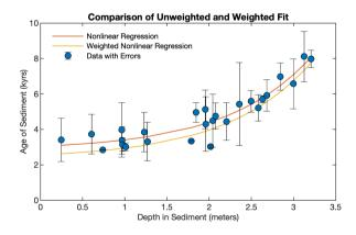
Comparison of unweighted (dashed line) and weighted (solid line) regression results from synthetic data. The plot shows the original data points (circles), the error bars for all data points, and the regression line for an exponential model function.
