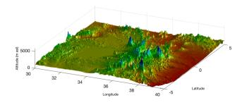
Surface plot of the GTOPO30 elevation data using light. The plot uses phong as the lighting type, which is very popular in 3D computer graphics and creates a combined diffuse and specular reflection on surfaces (data from the U.S. Geological Survey).
