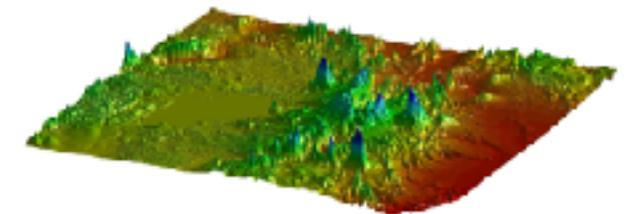
Surface plot of the GTOPO30 elevation data using light. The plot uses Phong as the lighting type creating a combined diffuse and specular reflection on surfaces.
